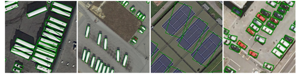
Figure 1: Some visualization results of Faster R-CNN towards oriented detection. It is obvious that the angle regression based method may lead to inaccurate results.
