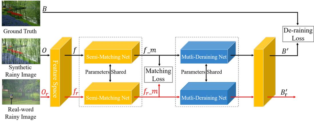
Figure 2: Multi-scale network structure based on semi-supervised learning
