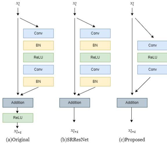
Figure 2: Comparison of residual blocks in original ResNet, SRResNet, and ours.
