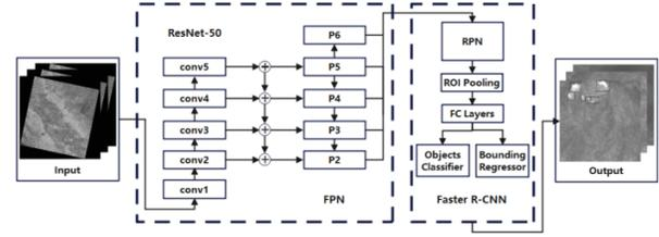
Figure 3: Faster R-CNN network structure with Resnet50+FPN as the backbone.
