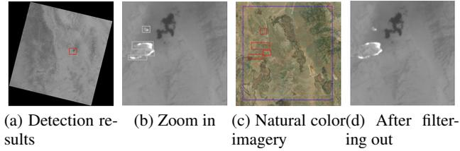
Figure 6: Nonwildfire area filtering for remote sensing imagery containing nonwildfire areas.
