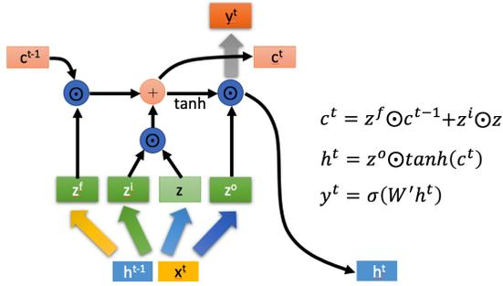
Figure 1: The internal structure of LSTM
