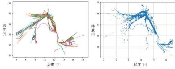
Figure 6: The DP algorithm obtains the compression result of the reference trajectory
