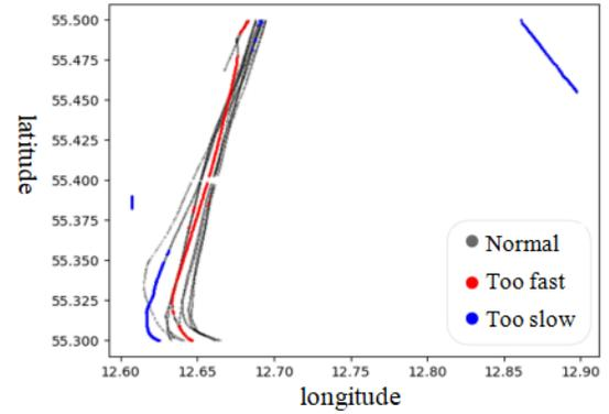
Figure 4: Determine the speed anomaly diagram
